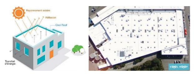
FIGURE 9 : SYSTÈME DE FONCTIONNEMENT (GAUCHE) ET TOITURE AYANT APPLIQUÉE LE REVÊTEMENT (DROITE)
