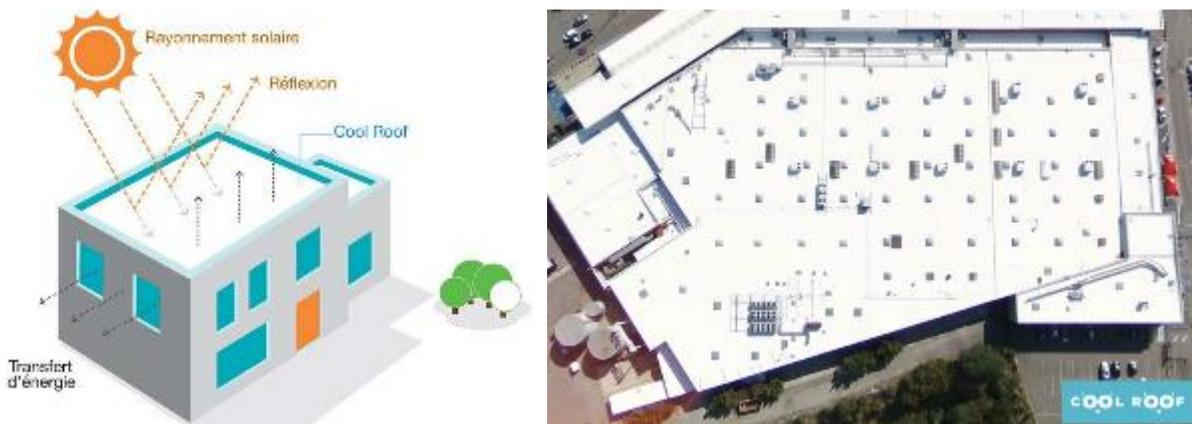
FIGURE 9 : SYSTÈME DE FONCTIONNEMENT (GAUCHE) ET TOITURE AYANT APPLIQUÉE LE REVÊTEMENT (DROITE)
